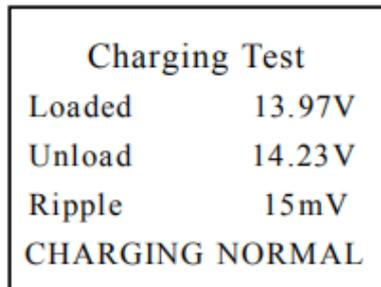
Check the connection between generator and battery, then retest.
