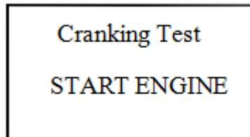
After entering the second start system test function ,the press OK key as following:Starting the engine as prompted, tester will automatically complete the cranking test and display the result.
